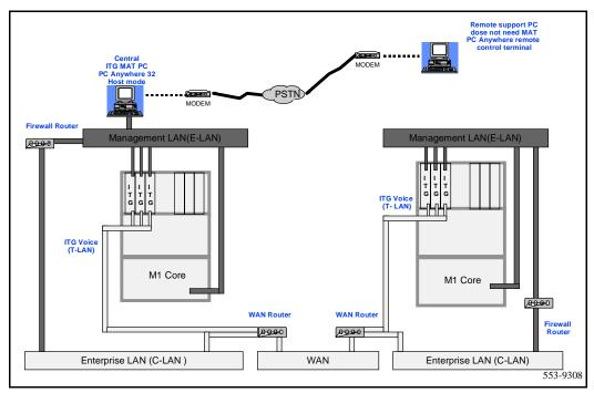
local and remote PCs. The local MAT PC is communicating with the ITG cards for management and alarm information and conveying all information back to the remote MAT PC. There are alternative solutions for remote alarm management available to the customer through third party products. The customer is referred to product bulletins for availability.
